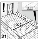
For unusual wall angles, you must first transfer the profile of the wall-line to the first row of panels and saw the panels accordingly. Measure the spatial dimensions of the room prior to installation. In the event that the first row of panels proves to have a width of less than 5 cm /  $2^{\circ}$ , you must then evenly partition the remaining length (excess length) among the first and last row of panels in such a manner that both rows are cut to size with the same (symmetrical) panel-width.
