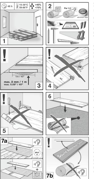
When installing onto a mineral sub-surface such as concrete, cement-screed, anhydritescreed or flagstone (among others), a moisture measurement must first be carried out. The following remnant-moisture levels in the screed may not be exceeded, prior to installation:
